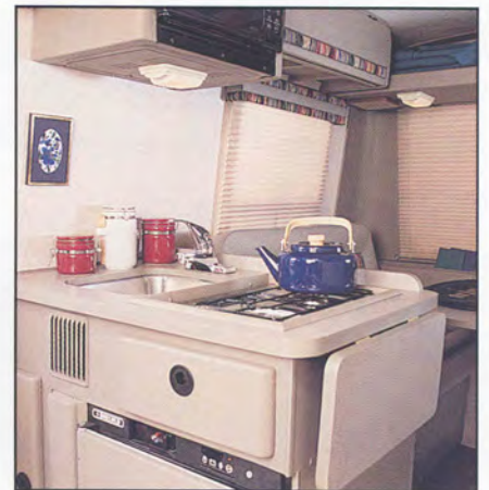
△ Kitchen appliances include a two-burner range top, refrigerator with three-way power source and an optional microwave.
