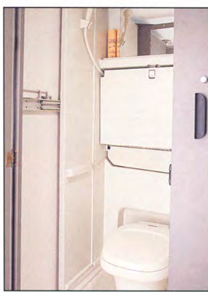
△ The bathroom features an ingenious telescoping wall system to provide privacy and an efficient use of space. Here the walls are shown extended.
