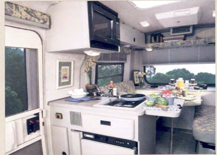
Quick fix. The galley features a two-burner recessed range top, microwave and stainless steel sink. A flip-up counter extension and drop-in sink cover add valuable work space to the galley area. The new skylight helps illuminate the galley.
