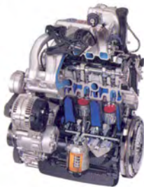
The 2001 Rialta is equipped with a 2.8 liter VR6 engine.
