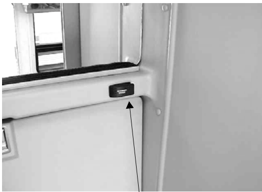
Shower Drain Pump Switch
