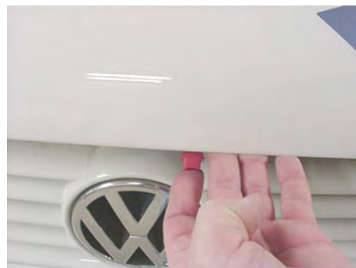
Push red 'Arrow' safety latch inward while lifting hood.
