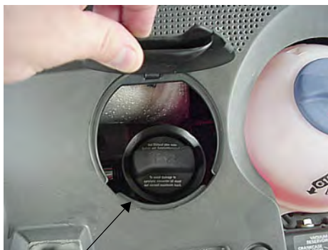
Engine Oil Fill Access
