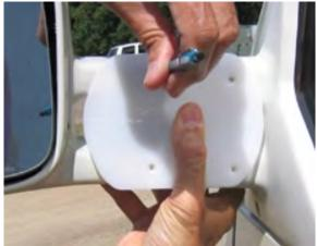
• Use center punch to dimple arms for correct drill location. Drill 4 holes in VW mirror mounting arms, 2 top, and 2 bottom. **Use !!!EXTREME CAUTION!!!**, when drilling the holes in the VW arms! The wires for your electric mirrors are located inside the hollow VW mounting arm. When drilling the holes, be very careful to not let the drill penetrate far inside the arm. It could cut or damage a wire and then the mirrors might not work.
