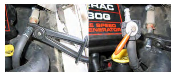
Cut the fuel line at the upper mark. Slip the clamp on the tube. Insert the top of the valve, slide the clamp down and release.
