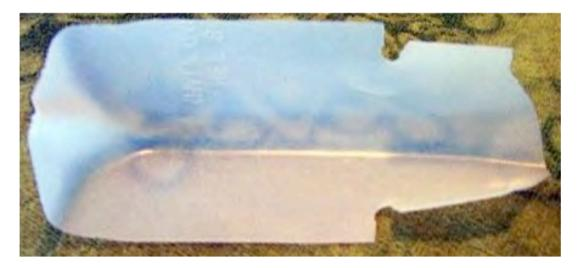
The smaller but wider funnel has relief slots on each side, which provide a slightly larger target for liquid, and the relief slots help insure the funnel is positioned well.
