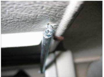
The pilot hole should be about 4 3/4" from the inside (hinged) side of the cabinet door. Again, place the screw through the spring, screw it in but do not tighten. Leave plenty of room for the spring to rotate on the screw.
