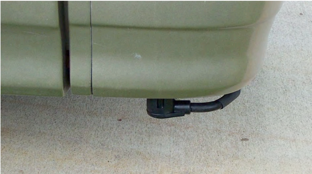
Generator 6 Ft extension cord with Female 30 Amp plug attached to the mounted 30 Amp Male plug [not visible] This is the configuration for driving, or for dry camping.
