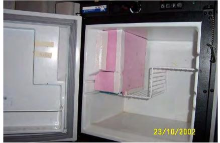
Freezer with door closed. Note: Styrofoam panels extend to the ceiling of the refrigerator and enclose forward cooling fins.
