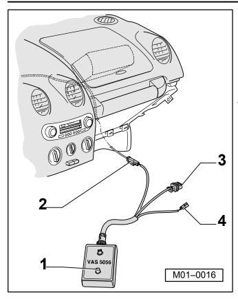
Airbag, connecting test box to front passenger airbag components, example
