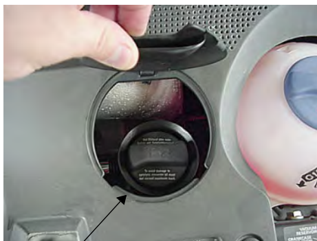
Engine Oil Fill Access
