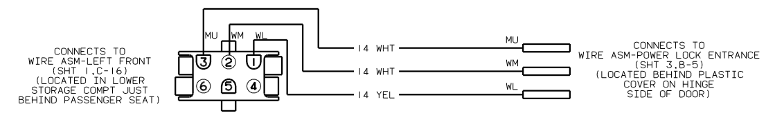
WIRING DIAGRAM-SIDEWALL (WIRE ASM 135846-01) 222HD & 222FD ONLY
