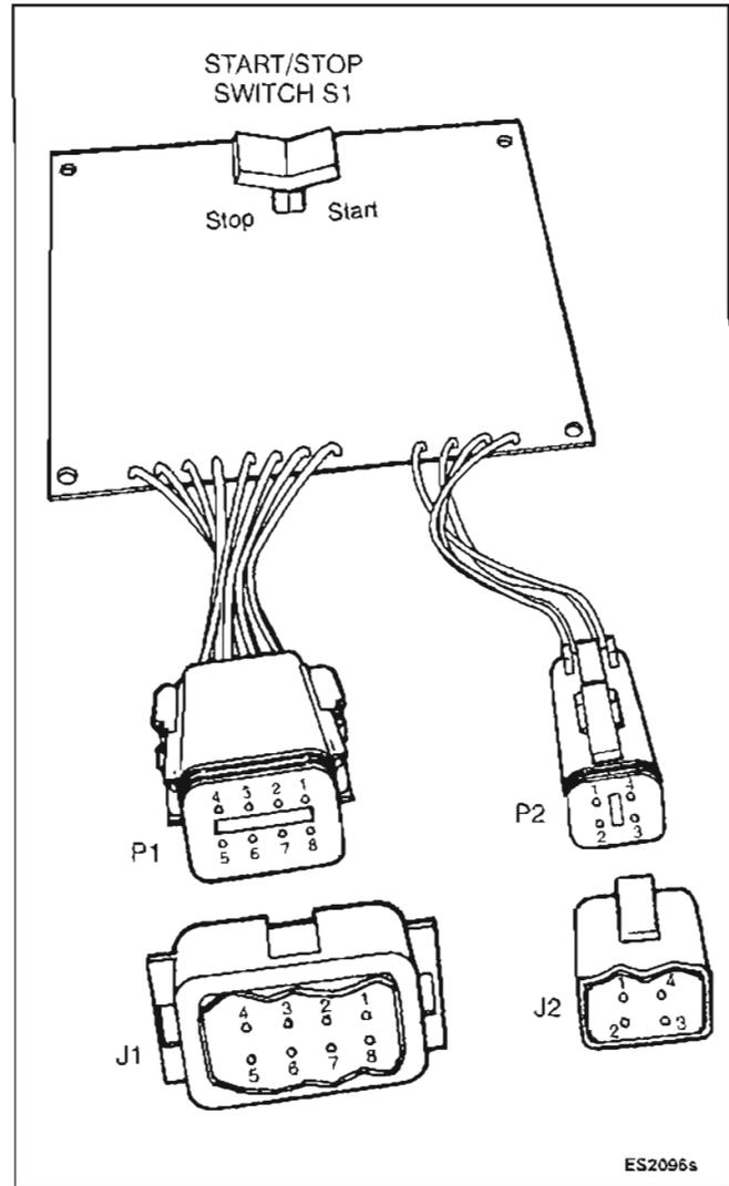
FIGURE 7-3. CONTROL ASSEMBLY (A1) – START/STOP SWITCH TEST
