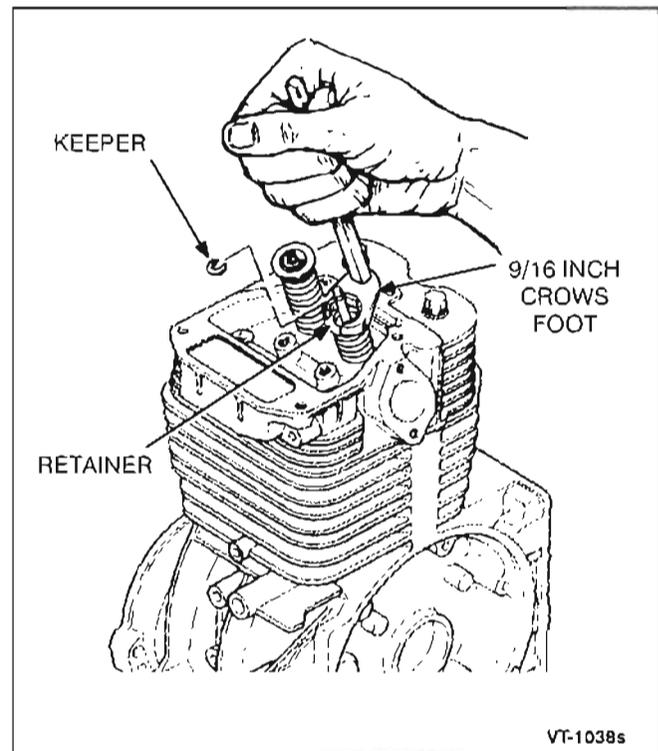
FIGURE 10-6. VALVE REMOVAL
