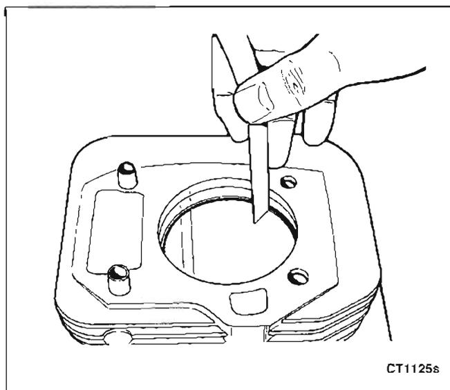
FIGURE 10-22. CHECKING RING GAP
