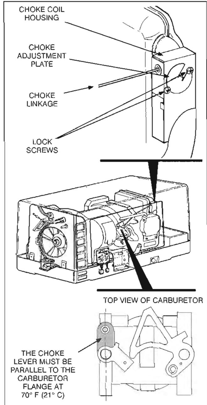
FIGURE 8-23. CHOKER ASSEMBLY (TYPICAL ALSO OF MODEL KVC)
