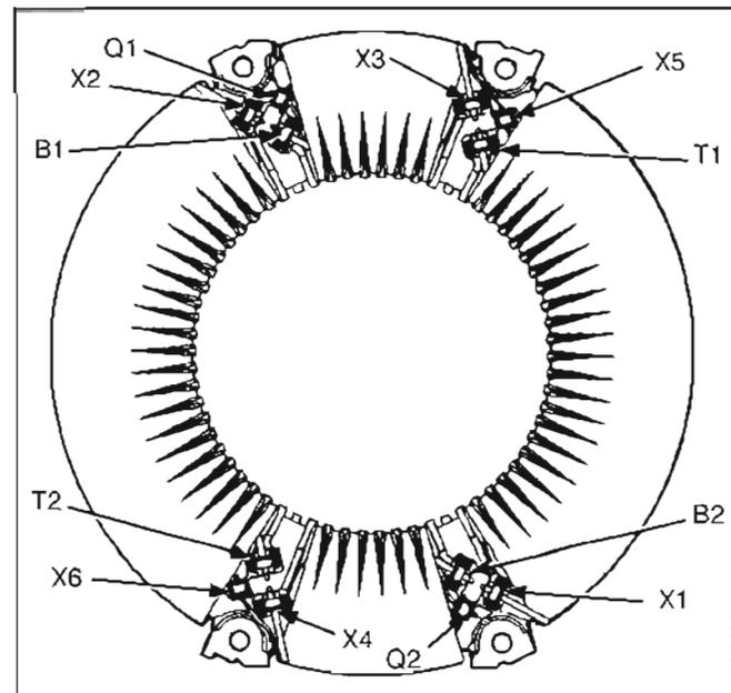
FIGURE 9-6. STATOR ASSEMBLY
