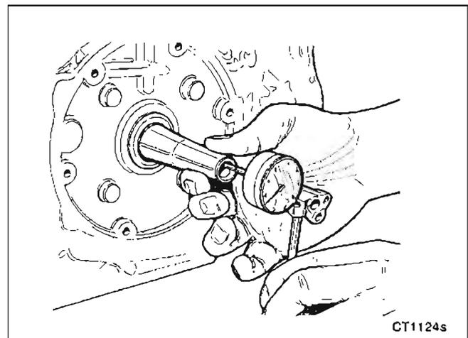
FIGURE 10-26. CHECKING ENDPLAY
