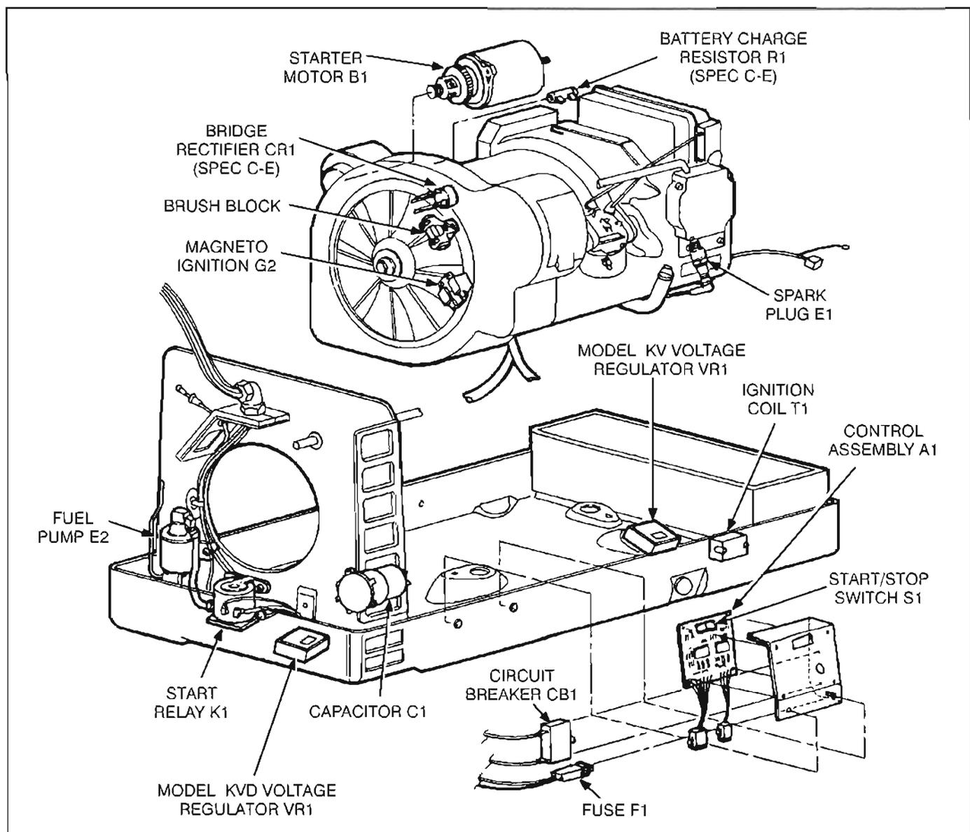
FIGURE 6-1. COMPONENT LOCATIONS (MODELS KV AND KVD)
