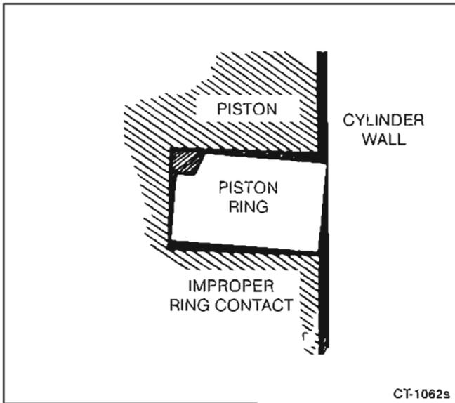
FIGURE 10-20. NEW RING IN WORN RING GROOVE
