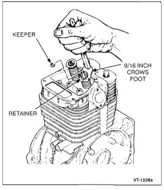
FIGURE 10-6. VALVE REMOVAL
