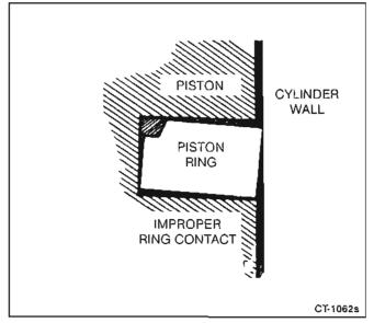
FIGURE 10-20. NEW RING IN WORN RING GROOVE
