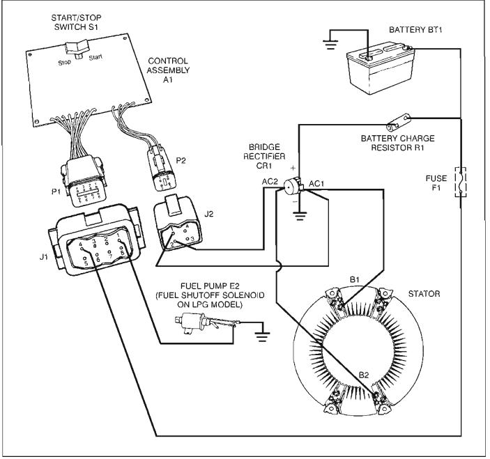
FIGURE 6-7. BATTERY CHARGE MODE (SPEC C – E)
