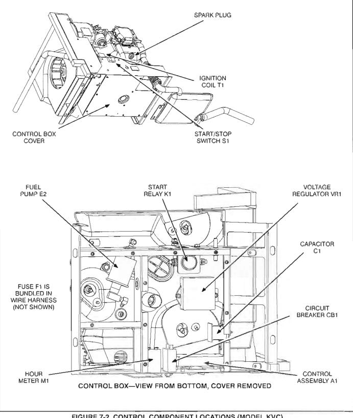
FIGURE 7-2. CONTROL COMPONENT LOCATIONS (MODEL KVC)
