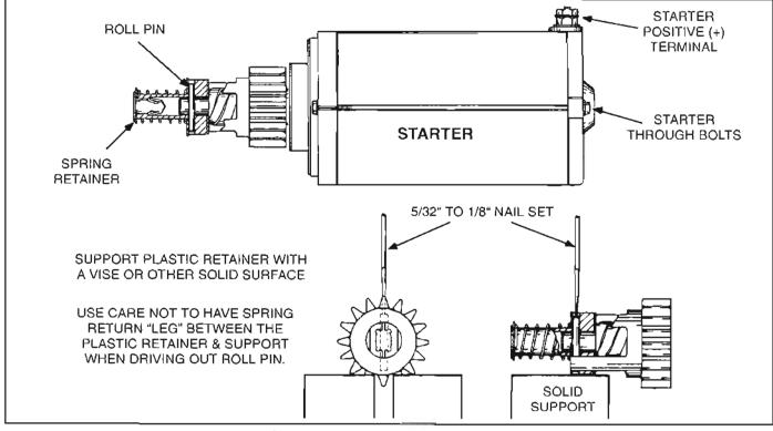
FIGURE 8-29. DRIVING ROLL PIN OUT
