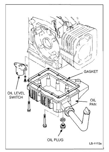
FIGURE 10-2. OIL PAN REMOVAL
