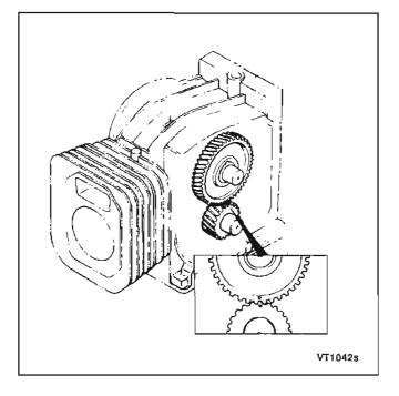
FIGURE 10-29. TIMING GEAR ALIGNMENT
