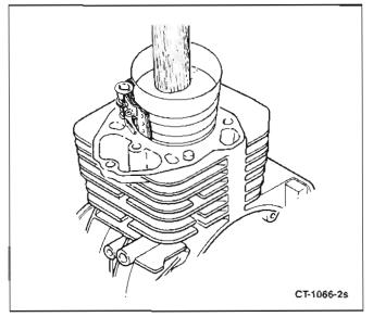
FIGURE 10-24. INSTALLING PISTON
