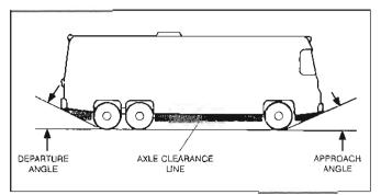
FIGURE 8-5. APPROACH AND DEPARTURE ANGLES AND AXLE CLEARANCE
