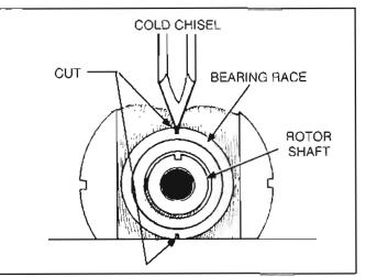
FIGURE 9-12, ROTOR BEARING REMOVAL
