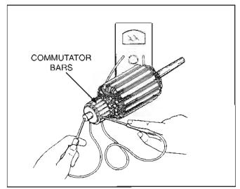
FIGURE 8-30. TESTING ARMATURE FOR GROUNDS
