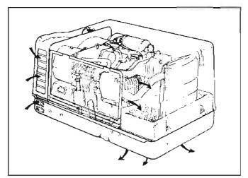
FIGURE 8-8. MODEL KV COOLING AIRFLOW
