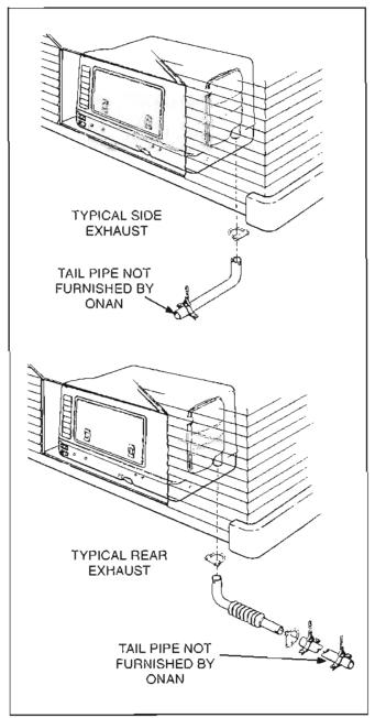
FIGURE 8-2. MODEL KV EXHAUST TAILPIPE
