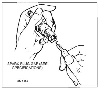
FIGURE 8-12. MEASURING PLUG GAP
