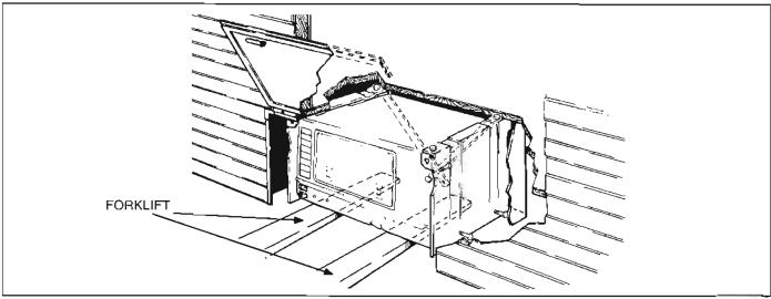
FIGURE 5-4, COMPLETE SET REMOVAL (MODEL KV)
