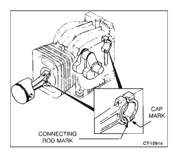
FIGURE 10-23. ROD CAP ASSEMBLY
