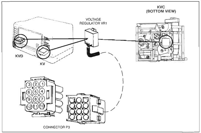
FIGURE 9-2. VOLTAGE REGULATOR LOCATION AND CONNECTOR P3
