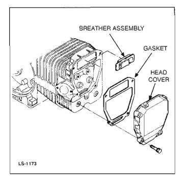
FIGURE 10-3. HEAD COVER REMOVAL
