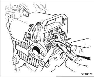
FIGURE 10-12. VALVE LASH ADJUSTMENT
