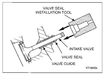
FIGURE 10-11. VALVE SEAL INSTALLATION
