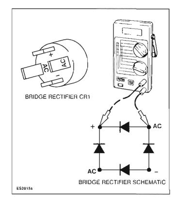
FIGURE 7-5. DIODE BRIDGE CR1 CHECK
