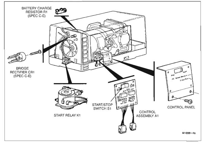
FIGURE 7-1. CONTROL COMPONENT LOCATIONS (MODELS KV AND KVD)
