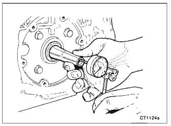
FIGURE 10-26. CHECKING ENDPLAY
