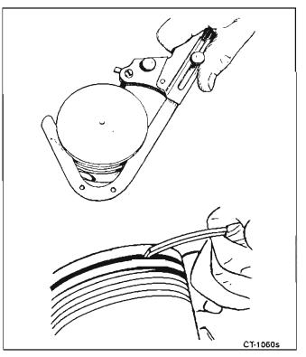
FIGURE 10-18. CLEANING RING GROOVES
