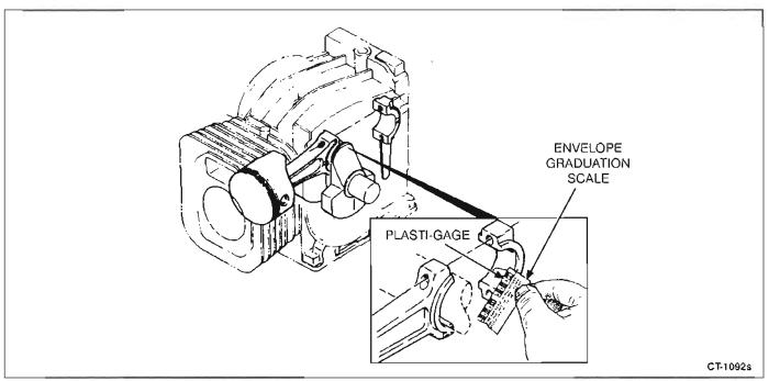
FIGURE 10-25. MEASURING CRANKPIN CLEARANCE
