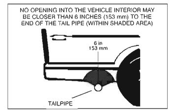
FIGURE 8-7. MINIMUM DISTANCES TO OPENINGS
