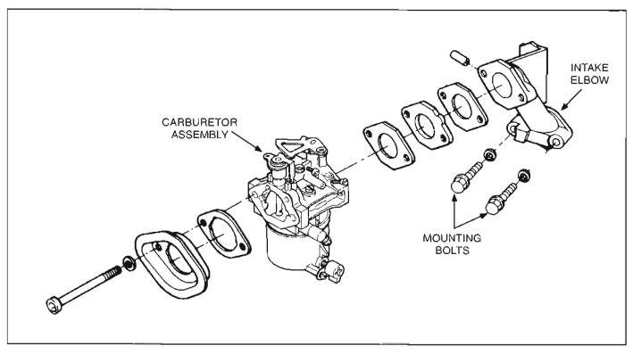
FIGURE 8-16. CARBURETOR AND INTAKE MANIFOLD ASSEMBLY
