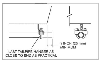
FIGURE 8-6. TERMINATING THE TAIL PIPE
