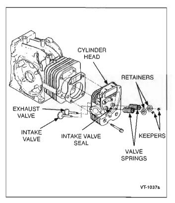
FIGURE 10-5. OVERHEAD VALVE SYSTEM
