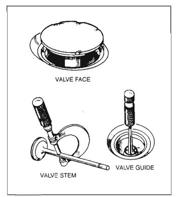
FIGURE 10-7. VALVE FACE, VALVE STEM AND VALVE GUIDE INSPECTION
