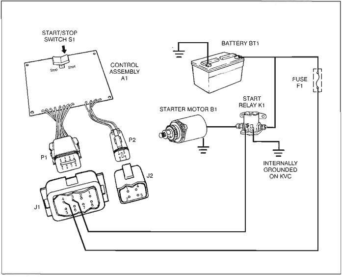
FIGURE 6-3. START – CRANKING MODE
