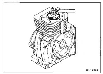
FIGURE 10-16. REMOVING WEAR RIDGE
