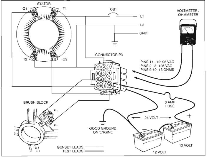
FIGURE 9-3. GENERATOR TEST SETUP AT HARNESS CONNECTOR P3
