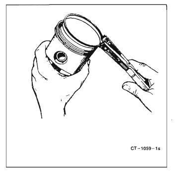
FIGURE 10-17. REMOVING PISTON RINGS
