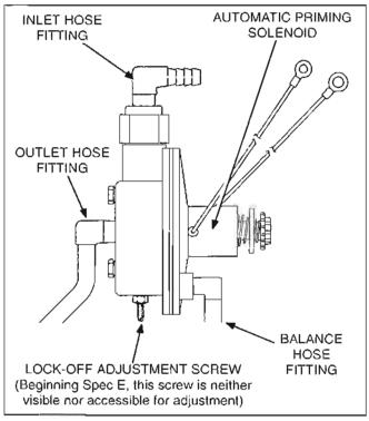
FIGURE 8-24. DEMAND REGULATOR WITH AUTOMATIC PRIMING SOLENOID
