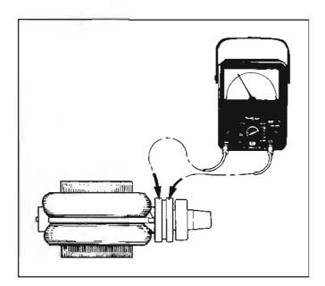
FIGURE 9-5. OPEN OR SHORTED ROTOR TEST
