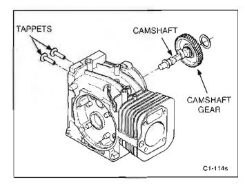
FIGURE 10-14. CAMSHAFT AND TAPPETS
