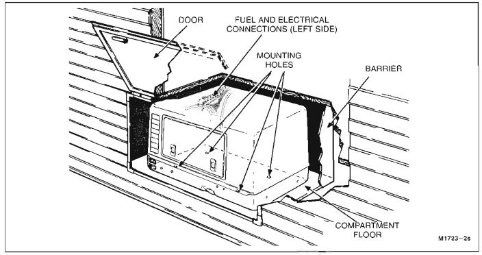
FIGURE 5-1. TYPICAL MODEL KV AND KVD COMPARTMENT INSTALLATION
