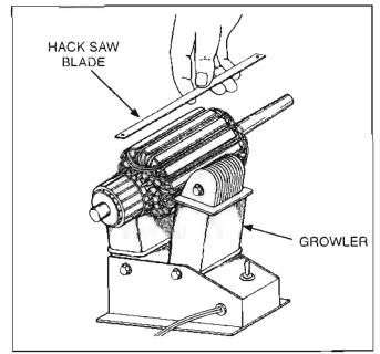
FIGURE 8-31. TESTING ARMATURE FOR SHORTS
