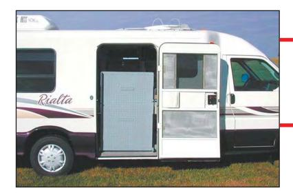
The Ability Equipped Rialta features a wide entrance door for wheelchair access. The convenient ramp folds up when not in use.
