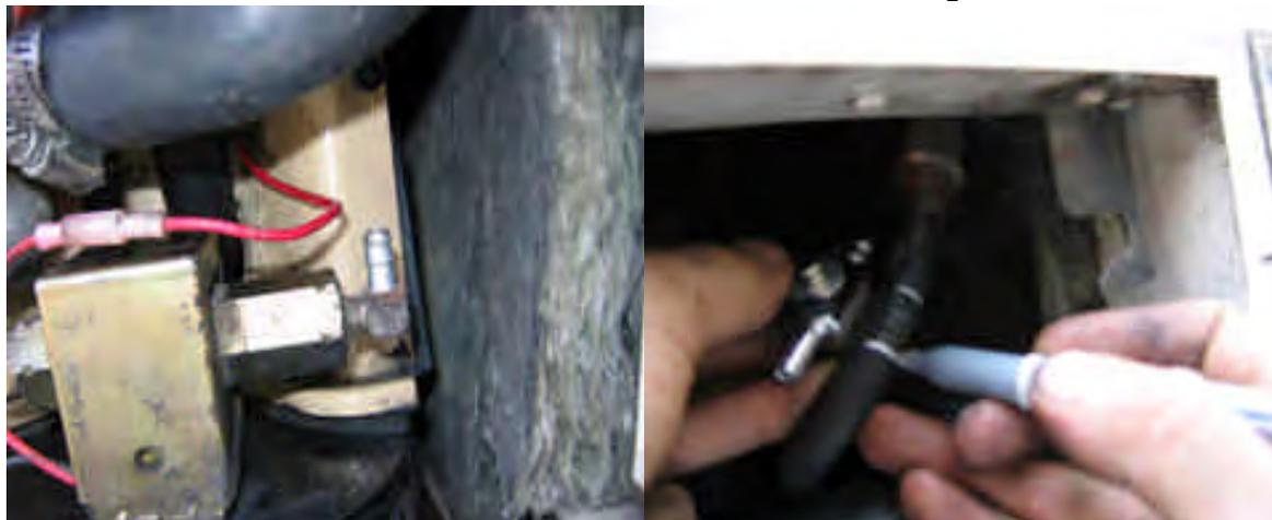
Clamp off the fuel line at the upper right. Cut the fuel line at the lower mark. Slip the clamp on the tube. Insert the bottom of the valve, slide the clamp up and release.
