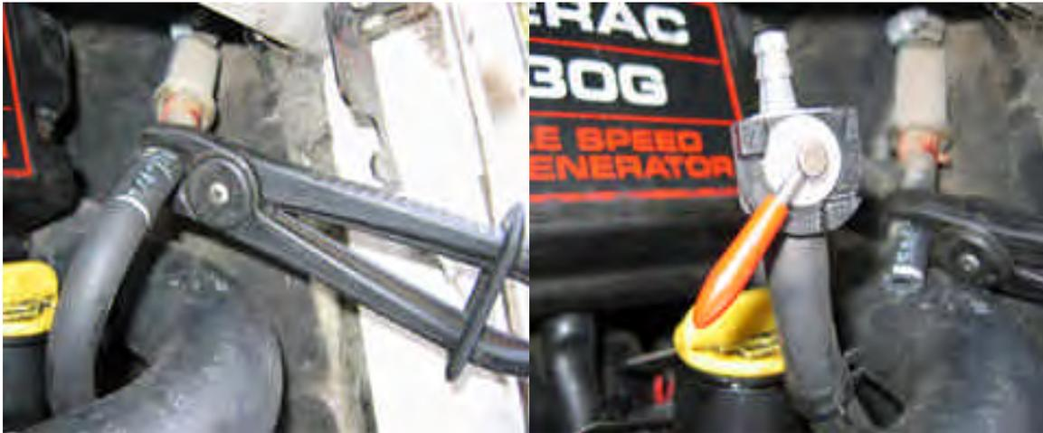
Cut the fuel line at the upper mark. Slip the clamp on the tube. Insert the top of the valve, slide the clamp down and release.
