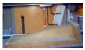
The finished ramps are 24 "long and while the overall height is about 5 3/4" the effective lift height is closer to 4". This is usually sufficient for slopes that are not too extreme. To store, the two ramps nest together and form a rectangle that will just fit in the outback storage area in the center section that is bumped out for the table in the HD and QD models. There should be additional room in the FD models.
