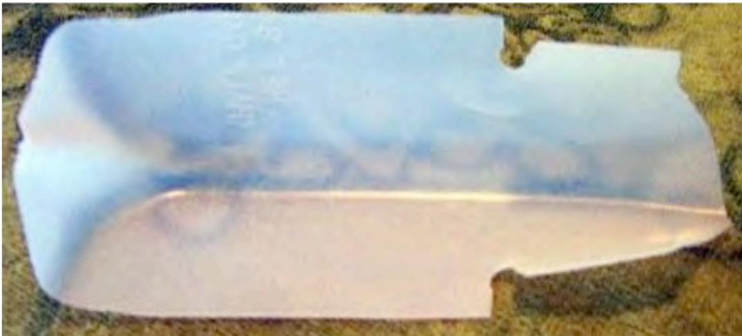
The smaller but wider funnel has relief slots on each side, which provide a slightly larger target for liquid, and the relief slots help insure the funnel is positioned well.
