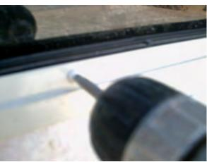
Remove all the screws holding the inside trim ring in place. Then remove the trim ring (it should just fall off after you remove all the screws).
