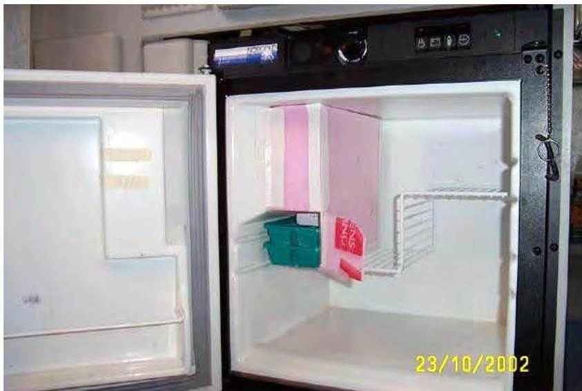
Freezer with door open. Two full-sized ice trays (4 1/4" x 10 3/4" with 14 cavities) fit nicely and freeze ice cubes overnight. Note: Although not obvious, the side panel does not go to the back wall, but instead, an aft panel fits between the aft fins of the cooling section, so the temperature sensor remains in the refrigerator compartment and not in the "Super Freezer" compartment. Also, the lower forward part is trimmed so as not to interfere with pop cans in the refrigerator door.
