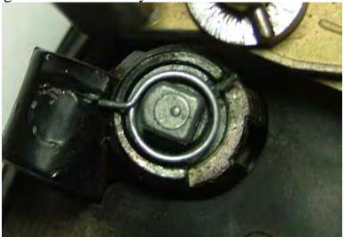
Use a small screwdriver to swing the end of the spring CCW to the notch.
