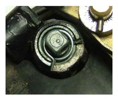
Be sure to put the key in the cylinder at this point so the wafers don't pop out when the cylinder is removed:
