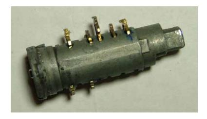
Remove the spring and carefully pull out the cylinder.
