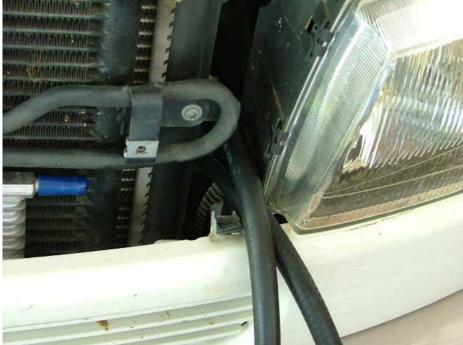
13. Notch filed in the plastic lower grill to allow the hose clamp to fit.
