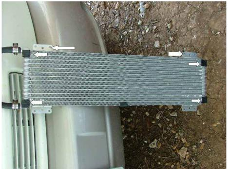
17. Cooler in place. End of hose clamp bent straight up to prevent contact with power steering cooler tube. I later added more padding at the top of the cooler fitting (arrow) to
