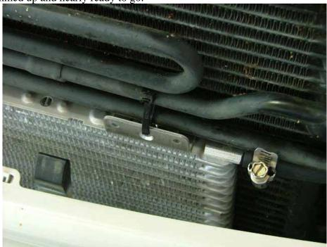
20. Water bypass coupling installed between hoses that were removed from the original cooler. Don't disconnect the water lines from the old cooler until you've got the Sonnax adapters installed to prevent the possibility of water getting into the transmission.
