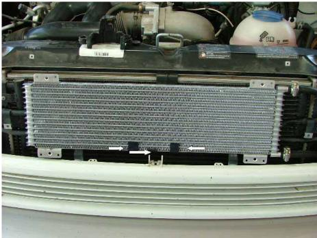
16. Locations of the pads on the back side of the cooler. I later added pads to the top brackets (top arrows) where the tie wraps were used to keep from rubbing the power steering cooler lines.
