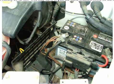
3. Battery left side cover panel removed. It pulls straight up out of the notches of the battery box frame. You can barely see one of the Banjo bolts at the arrow. This is the room you have to work with when you do the installation. It will be mostly one-handed and mostly by touch.
