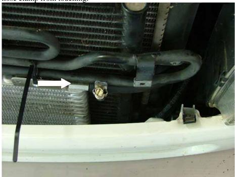
18. Tie wraps installed to hold cooler in place.
