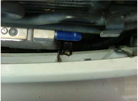
15. Both hoses attached to the cooler before sliding into place. Note pads on front to prevent metal-to-metal contact. By leaving a little extra hose, the cooler can be pulled out and moved off to the side. This would be needed when changing spark plugs and the radiator has to be tilted forward.
