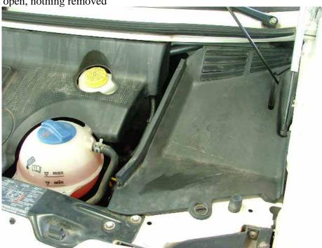
2. Main battery cover off. You may have to pull the cable brackets loose on the left side.
