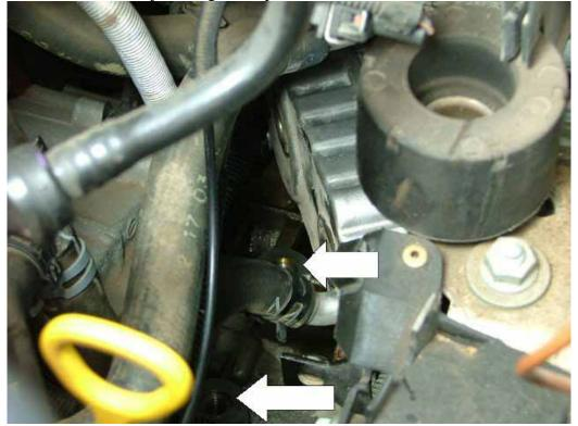
11. Sonnax adapters installed. I had the best luck installing the one toward the rear of the vehicle first. The real trick is to get the Banjo bolt through the adapter and get it started into the hole without moving the o-ring in the groove. If you begin to get a little frustrated, take a short break and try again. The adapter closest to the back of the vehicle (top in this picture) goes to the top of the cooler and is the output from the transmission.
