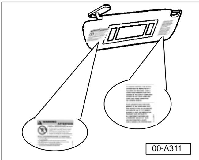
◀ New labels are located on either side of sunvisor mirror (sunvisor flipped down) as shown.
