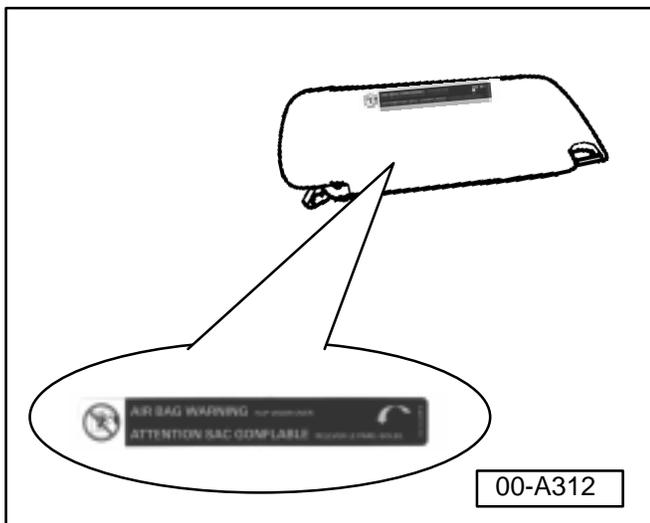
◀ A new label is located on sunvisor (sunvisor flipped up) as shown.
