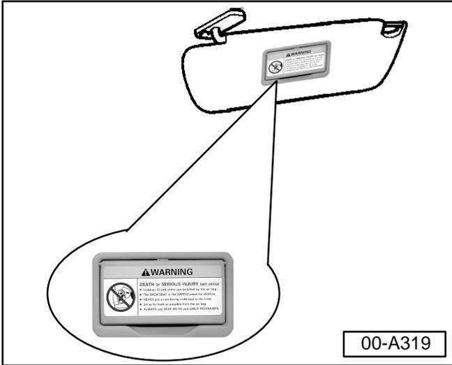
Labels are located on each sun visor mirror (sun visor flipped down) as shown.
