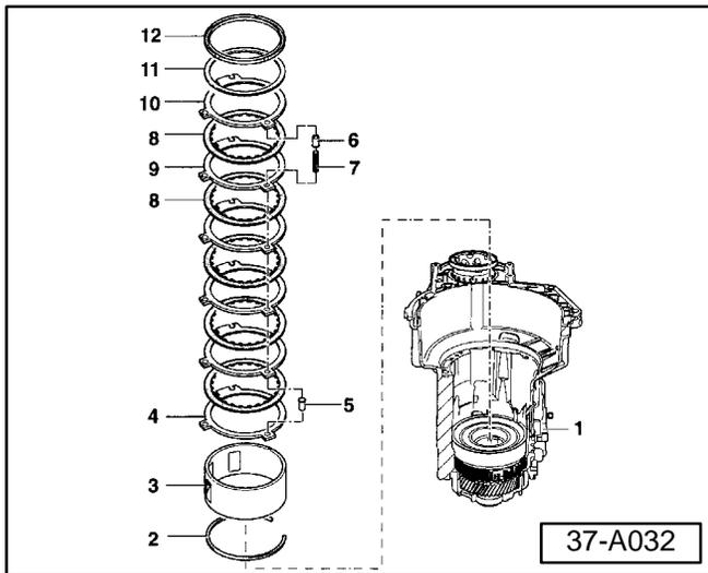
◀ The two rings that fit into the round ring -2- touch on the outside edge and are apart on the inside edge (effect allows rings to act like a spring).
