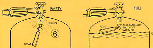
Fig. 3 The OPD Valve helps prevent overfilling of LP-gas in the container.
