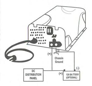
CAUTION:OBSERVE POLARITY WHEN CONNECTING BATTERY(S), REVERSE POLARITY WILL BLOW CONVERTER OUTPUT FUSES.
