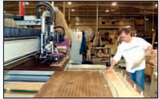
*With this machine an operator can set up one job while the automated router is working on another project.*
