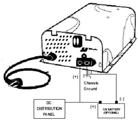
CAUTION: OBSERVE POLARITY WHEN CONNECT-ING BATTERY(S). REVERSE POLARITY WILL BLOW CONVERTER OUTPUT FUSES.
